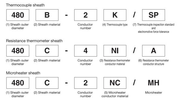
(1) Sheath outer diameter: A value that is 100 times the sheath outer diameter (examples: "480" for a diameter of 4.8 mm and "050" for a diameter of 0.5 mm)
